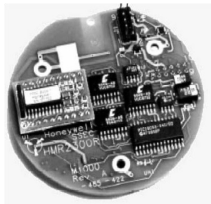
图1 HMR2300R 3轴捷联式磁力计及载板
